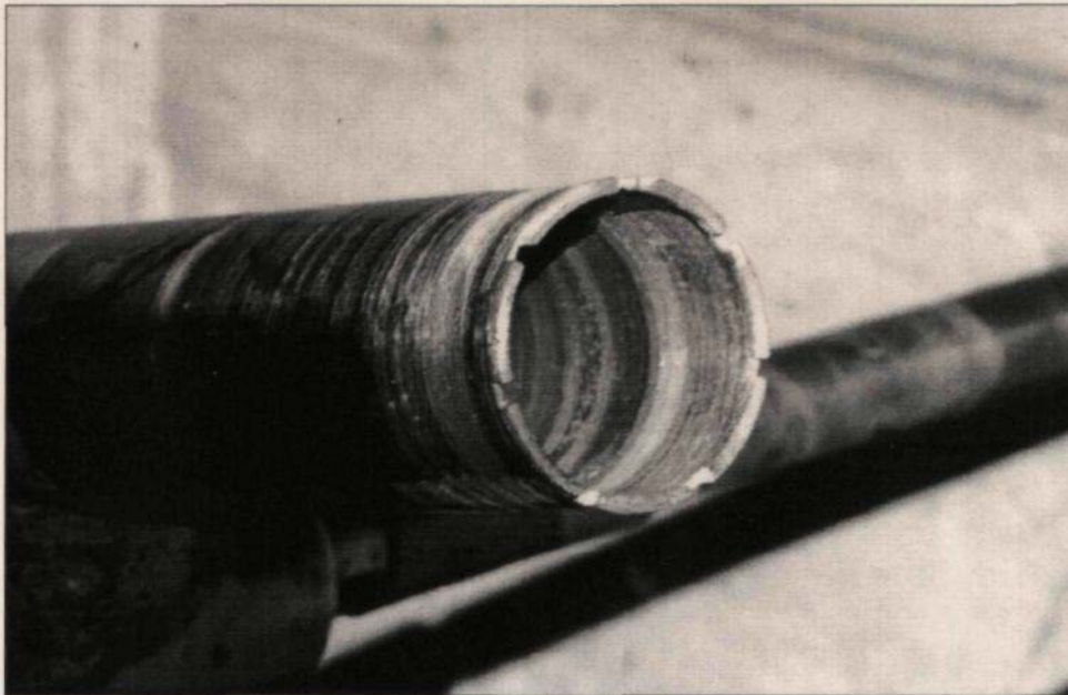
This diamond embedded rotary drill is a commonly used tool.
